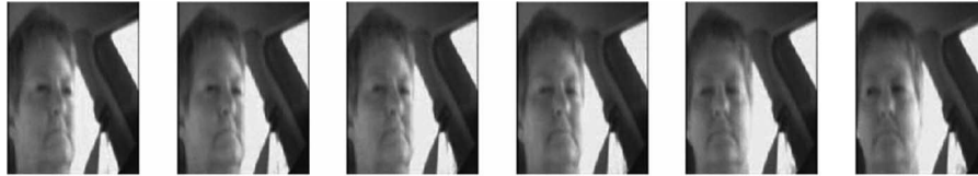
Fig. 14. Sequence of frames which shows subject 46 moving from Pose 3 to Pose 7 . The ground truth for this sequence was determined to be [3, 3, 3, 3, 7, 7], and the classifier output for this sequence was [3, 3, 3, 6, 7, 7].
